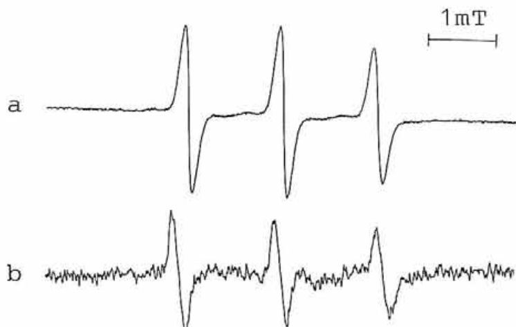
FIGURE 7 a ) The EPR spectrum obtained by the decomposition of S-nitroso-N-acetyl-D,L-penicillamine (1 mM) in the presence of 10 mM DBNBS ( a_N = 1.40 mT). b ) The EPR spectrum obtained by the DBNBS trapping of glutathionyl radical ( a_N = 1.42 mT). The concentration of DBNBS was 50 mM. Glutathionyl radical was generated by the following two methods: (1) the mixing of glutathione (10 mM), H_2O_2 (2 mM), horseradish peroxidase (0.2 mg/ml). (2) the reaction of glutathione (50 mM) and isoamyl nitrite (50 mM).
